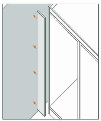
The side scribe is fitted BEFORE the top plinth is fitted
