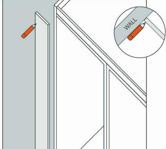
If the wall is too far out of square the pencil may fall off the edge of the panel. If this is the case then use a pair of compasses or wrap tape around the shaft of the pencil to make it thicker.
